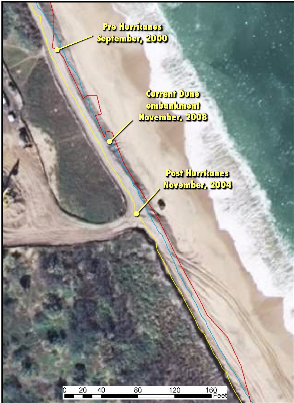
Figure 12. Barrier Island Sanctuary Dune Loss Due to Hurricane Frances and Jean.
